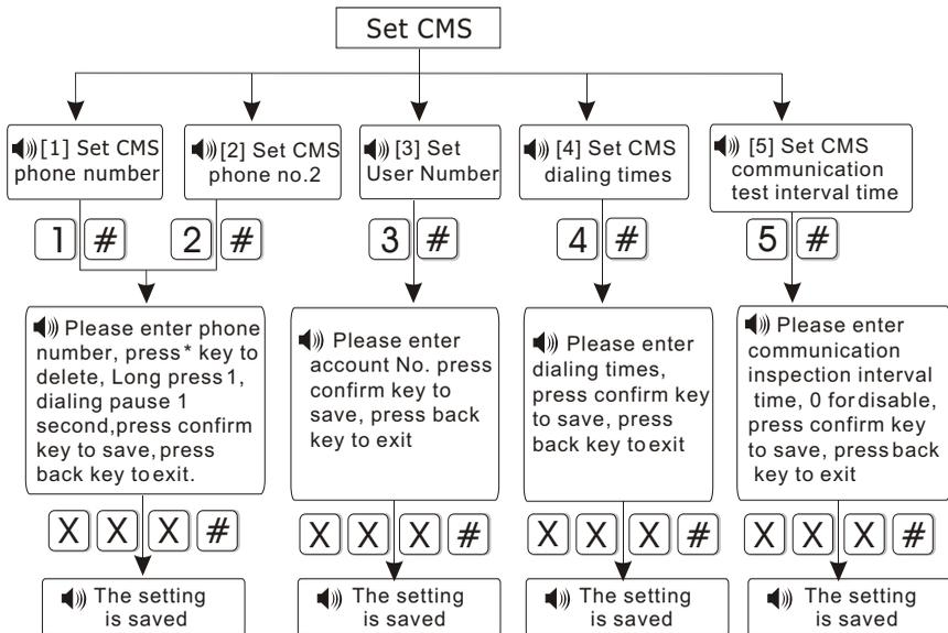
Note: 1.The user code is the identification code in CMS setting, CMS 1 and CMS 2 use the same user code; dialing times can be set 1-15 , communication inspection interval time can be set 0-999 hours, the common setting is 24 hours.
