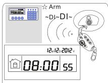
Press the keyfor arm awayon remote or the keypad,then you hear"system armed,please exit the protection area" there will be "Dee-dee" sound to confirm the system is armed successfully.
