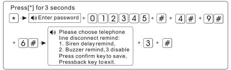
6.4.9.7 set zone alrm times: if set the alarm alarm times as 1, when zone start alarm but the zone is trigger one time again, the panel will not make alarm.
