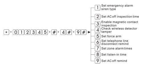
6.4.9.1 Set emergency alarm siren type( the default setting is mute) For example: set emergency alarm siren type is pedal point.
