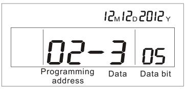
Press key up and down to check and modify the different data of the data bit.
